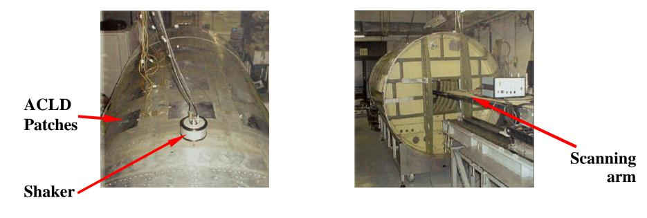
Fuselage, Shaker & Control Patches
