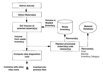
Fig. 3. Modeling process for treating disposition of wastes in the waste inventory. A "remnant" is a portion of the original waste material that is tagged to indicated that a waste disposition activity has been performed on it.
