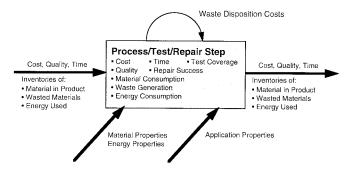
Fig. 4. General process step model used within the SavanSys software tool.
