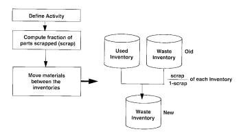
Fig. 2. Modeling process for defective parts that are scrapped as a result of inspection or test activities. scrap is the fraction of panels or boards scrapped by the test or inspection step.
