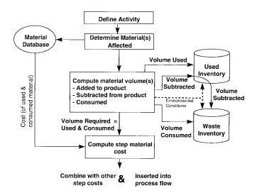
Fig. 1. Modeling process for treating material addition and subtraction. The environmental conditions are necessary to convert the material volumes to STP. The material database provides material cost and waste disposition information.
