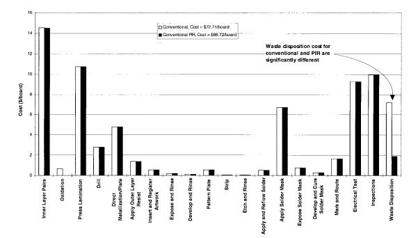
Fig. 9. Cost of conventional and PIR full multilayer build including waste disposition. (The actual process models used consist of  $\sim$ 230 process steps that have been combined in this figure of convenience.)
