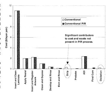
Fig. 8. Cost of conventional and PIR layer-pair fabrication including oxide treatment, excluding waste disposition. (The actual process models used consist of  $\sim$ 30 process steps that have been combined in this figure for convenience.)
