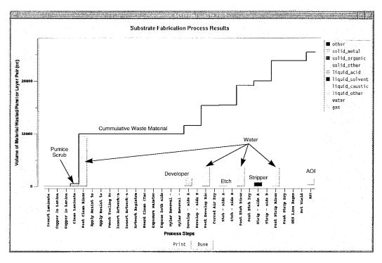
Fig. 7. Material wasted as a function of the process steps associated with fabricating a double-sided, undrilled, copper clad layer-pair.
