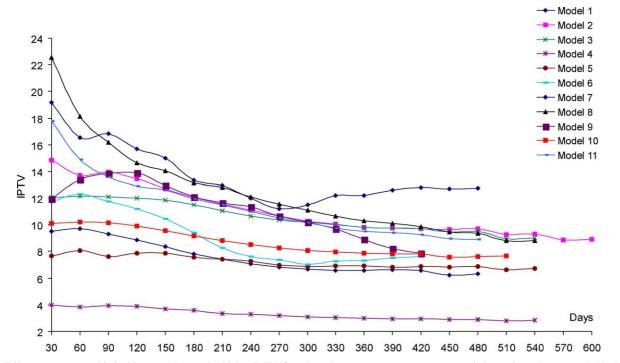
Fig. 2. Failure rates expressed in incidents per thousand vehicles (IPTV) for selected passenger compartment mounted electronic products recorded by Delphi Corporation. The actual IPTV values have been modified to protect the proprietary nature of the data.
