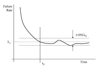
Fig. 3. Change point estimation for  $t_S$ ,  $\lambda_S$  is the failure rate at  $t_S$ .
