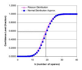
**Figure 6.6.** Sparing calculation for n = 25000, t = 1500 hours, and  $\lambda = 0.5$  failures/million hours
