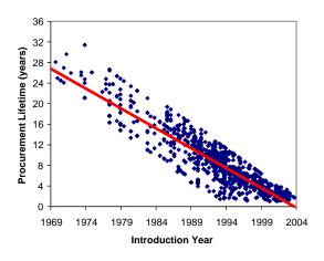
**Figure 6.9.** Decreasing procurement lifetime for operational amplifiers, [6.25]. The procurement life is the number of years the part can be procured from its original manufacturer
