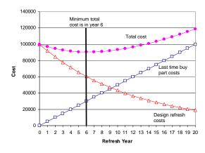
Figure 6.12. Example application of Porter's refresh costing model
