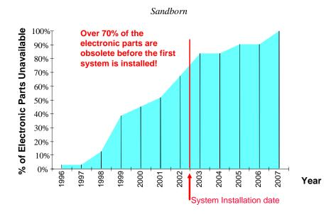
Figure 2: Percent of Commercial Off The Shelf (COTS) parts that are out of production (unprocurable) versus the first 10 years of a surface ship sonar system's life cycle (courtesy of NAVSURFWARCENDIV Crane)
