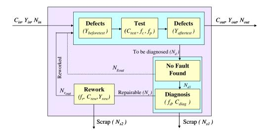
Figure 1. Test/diagnosis/rework (TDR) model from Trichy *et al.* (2001). Table 1 describes the notation appearing in this figure.
