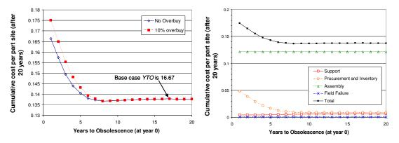
Figure 6. Cumulative cost per part site as a function of part procurement life (*YTO*) for (left) 0% and 10% overbuy on lifetime buys, and (right) 10% overbuy with respect to cost category.
