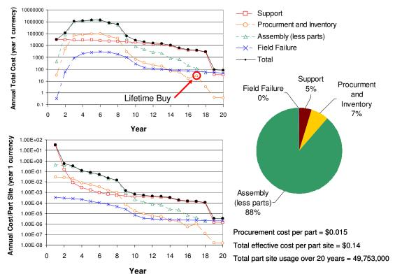
Figure 3. Example part total cost of ownership modeling results (high-volume case).
