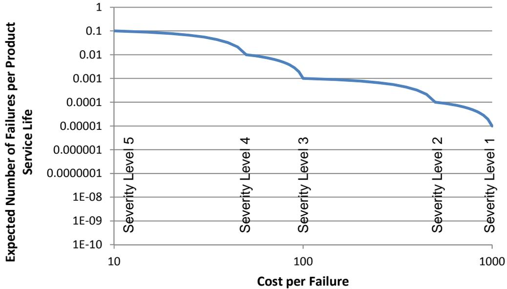
**Fig. 3.** Expected number of failures vs. cost per failure.
