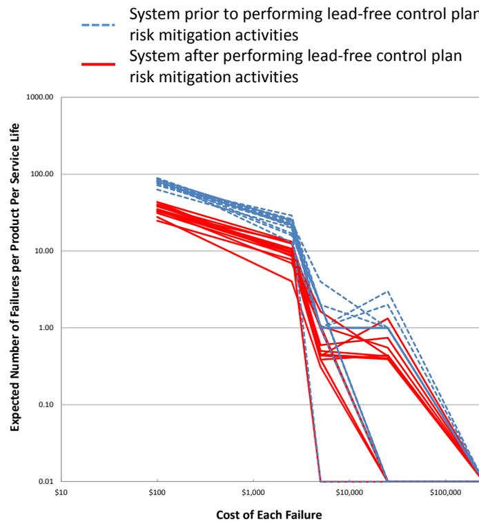
Fig. 12. Results for the commercial aircraft,  $\eta = 50,000$  cycles.
