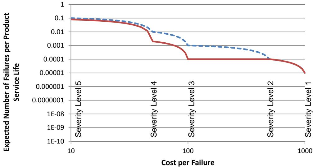
**Fig. 4.** The blue (dashed, top) curve represents the number of failures per product per unit lifetime at each severity level before activities are considered, and the red (solid, bottom) line represents the expected number of failures with the activities performed.
