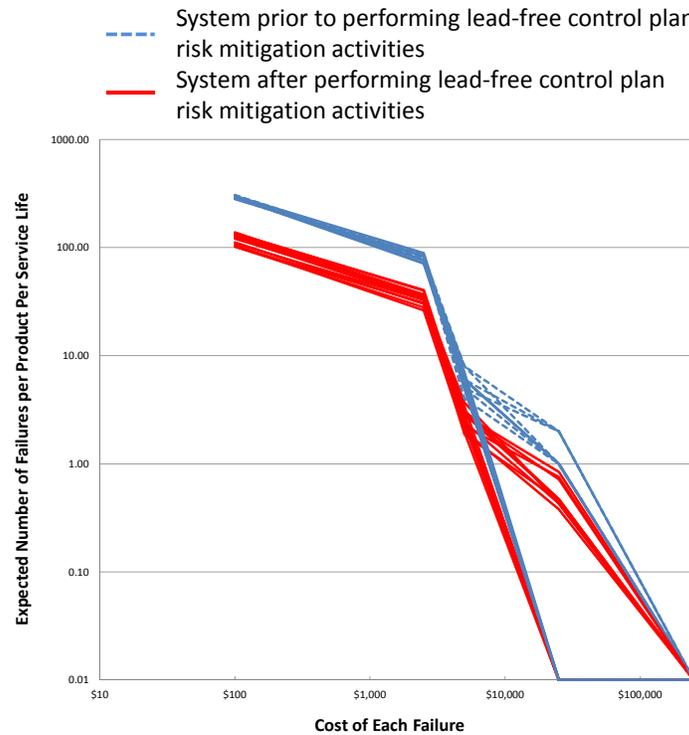
Fig. 10. Results for the commercial aircraft,  $\eta = 25,000$  cycles.
