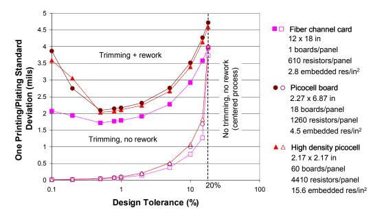
Figure 3 – Application-specific economical regions of trimming and reworking embedded resistors. This example result assumes no resistor thickness variation, see [13] for additional assumptions and modeling parameters associated with this result.
