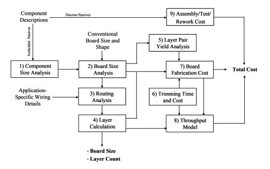
Figure 1 – Embedded passive board cost tradeoff model [8].
