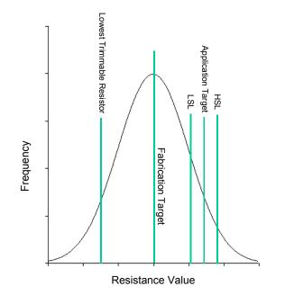
Figure 2 – Distribution of fabricated resistor values.
