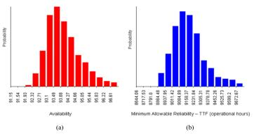
**Figure 3:** (a) Required Availability Distribution; (b) Computed Minimum Allowable Reliability (*TTF*) in Operational Hours, for an Unscheduled Maintenance Policy
