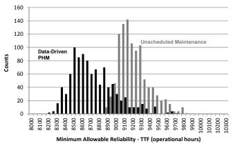
**Figure 4:** Computed Minimum Allowable Reliability (*TTF*) Distribution for Unscheduled Maintenance and Data-Driven PHM to Meet an Availability Requirement. Both Maintenance Approaches Satisfy the Same Availability Requirement.
