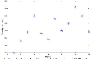
Figure 1. Capacity factor in a Kansas wind farm August 2007 to June 2008 (http://kcc.ks.gov/energy/chart.htm)
