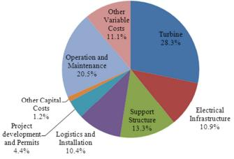
Figure 3. Projected life cycle cost breakdown for offshore wind turbines
