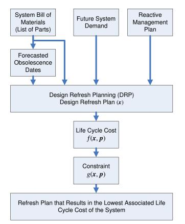
Figure 1. DESIGN REFRESH PLANNING (DRP) PROCESS SHOWING THE REQUIRED INPUT DATA AND THE RESULTING OUTPUT.
