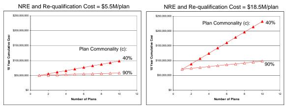
Figure 5 - The 10 year cumulative cost of different quantities of plans supported by the supplier as a function of the plan commonality. NRE and qualification cost: Left = \$5.5 million/plan, Right = \$18.5 million/plan.
