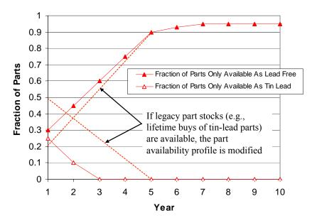
Figure 1- Fraction of parts available only as tin-lead or lead-free.
