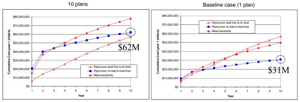
Figure 4 - Effect of the number of different plans supported by the supplier. Left = 10 plans, Right = 1 plan. 65% commonality between plans assumed.
