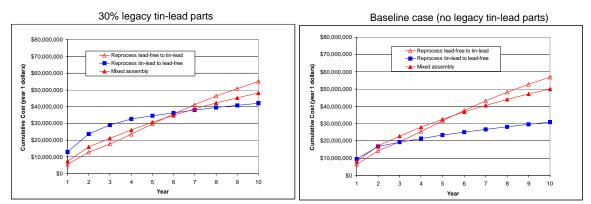
Figure 6 - Effect of tin-lead part availability on cumulative cost for 1 plan. Left = 30% tin-lead legacy parts, Right = baseline part availability profile.
