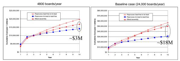
Figure 3 - Effect of board production quantity on cumulative costs. Left = 4800 boards/year, Right = 24,000 boards/year.
