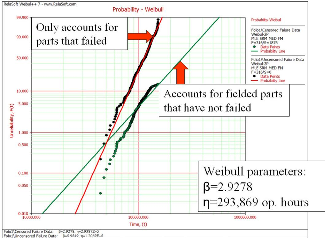
Fig. 7 Part number 5004-02 failure distribution. Both data sets are equal, one shows 10% unreliable, the other 100% unreliable (censored vs. uncensored).
