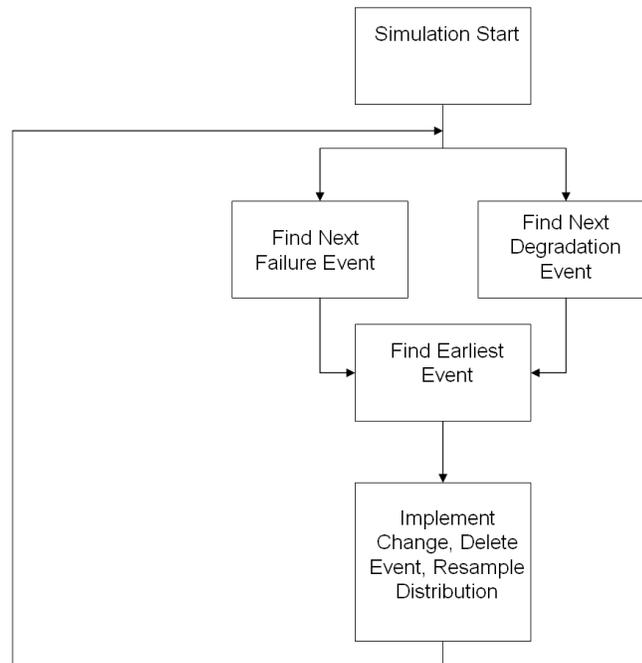
Fig. 3 Discrete-event simulation flow for multiple events
