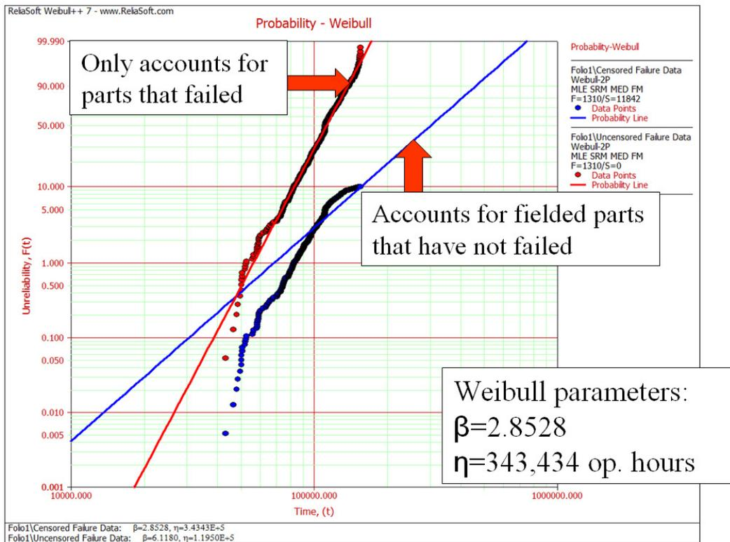
Fig. 6 Part number 3798-05 failure distribution. Both data sets are equal, one shows 10% unreliable, the other 100% unreliable (censored vs. uncensored).
