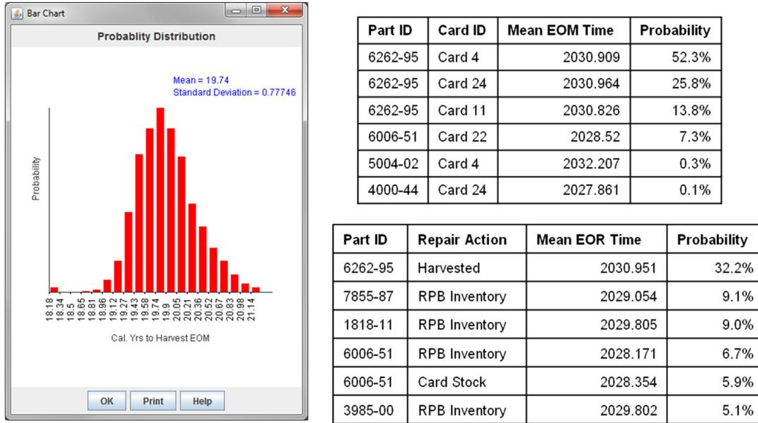
Fig. 10 System-level EOM distribution (left), EOM (top right) and EOR (bottom right) results for Case 3
