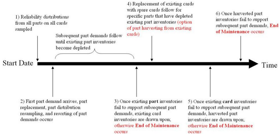
Fig. 1 EOR/EOM part failure process flow
