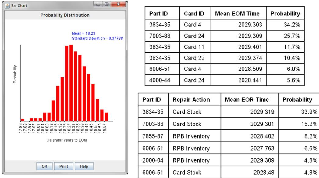
Fig. 9 System-level EOM distribution (left), EOM (top right) and EOR (bottom right) results for Case 2
