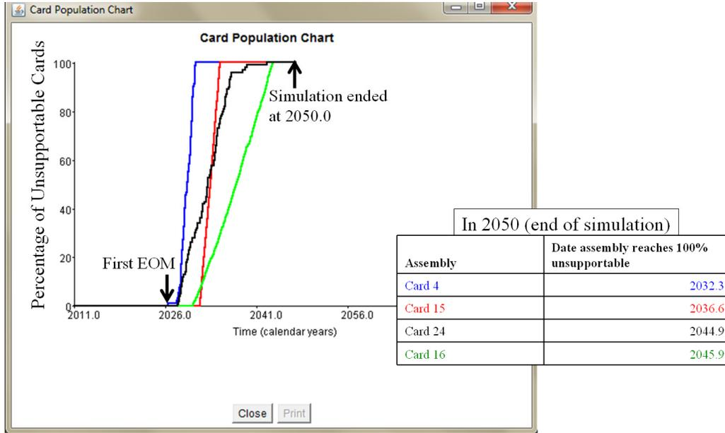
Fig. 11 Card-level support tracking and loss
