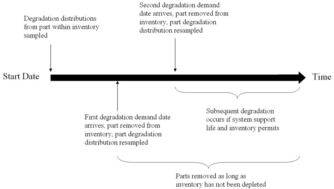
Fig. 4 Part degradation process flow
