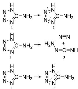
**5-Aminotetrazolium Dinitramide.** The cation of 5-aminotetrazolium dinitramide (HAT\_DN), 5, contains the basic aminotetrazole structure and is paired with the dinitramide ( $\text{N}_3\text{O}_4^-$ ) anion. Of the materials studied, this has the slowest reaction time (Table 1), which allows for the capture of multiple steps within the reaction that may not be detectable for other materials. Figure 1 is a single detailed
