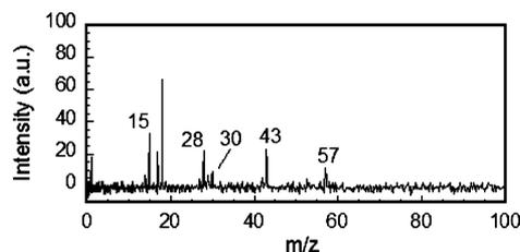
**Figure 6.** Detailed mass spectrum of the reaction products from heating of MeDAT\_N3, 12.
