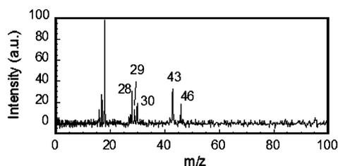
**Figure 7.** Detailed mass spectrum of the reaction products from heating of DAT\_N, 13.
