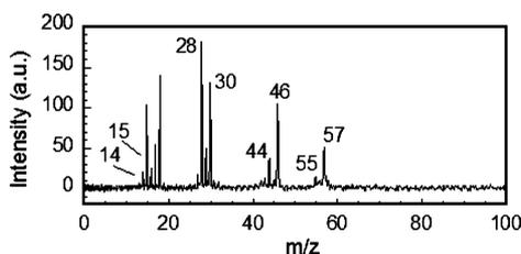
**Figure 3.** Detailed mass spectrum of the reaction products from heating of MeDAT\_DN, **11**.
