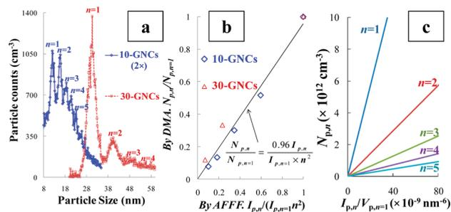
**Figure 3.** Comparison of AFFF and ES-DMA. (a) Particle size distributions from ES-DMA for the same samples analyzed by AFFF in Figure 1a. (b)  $N_{p,n}/N_{p,n=1}$  (measured by ES-DMA) versus  $I_{p,n}/I_{p,n=1}$  measured by AFFF (normalized by  $n^2$ ). Diamonds, 10-GNCs; triangles, 30-GNCs. (c) Calculation of  $N_{p,n}$  of GNCs from  $I_{p,n}$  using eq 2.  $n$  ranges from 1 to 5.
