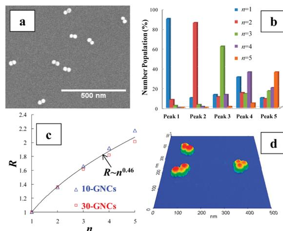
**Figure 2.** FE-SEM and AFM analysis of 30-GNCs fractions resolved by AFFF. (a) FE-SEM image of peak 2 fraction in Figure 1a. Scale bar is 500 nm. (b) Histograms generated from FE-SEM images. (c)  $R$  vs  $n$  curve is the power law fit to triangles and squares representing experimental data of 10-GNCs and 30-GNCs, respectively. (d) AFM image of peak 3 fraction in Figure 1a. The height ( $z$  direction) scale is from 0 to 30 nm.
