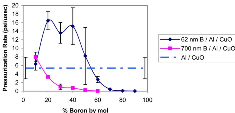
Fig. 2. Experimental pressurization rate as a function of % boron in an Al/B/CuO MIC for both nano- and micron-sized boron. The horizontal line is Al/CuO data, included for comparison. Error bars represent the standard deviation of the experimental data.
