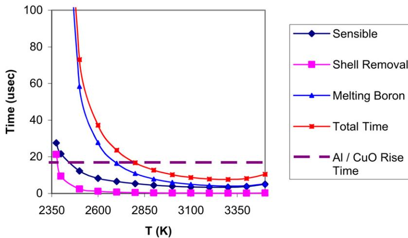
Fig. 7. Model predictions of the timescales as a function of surrounding temperature for a 700 nm boron particle.
