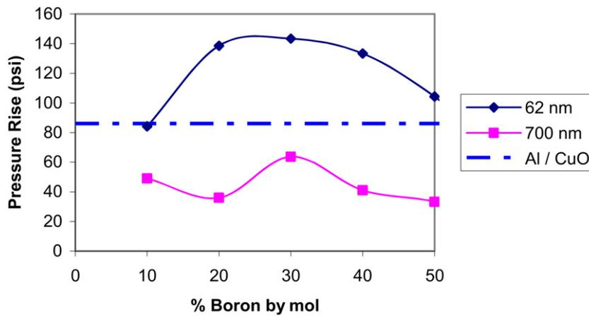
Fig. 5. Experimentally measured pressure rise in the region where an enhanced reactivity is observed (<50% B by mol).
