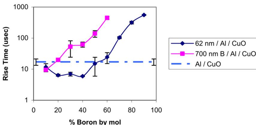
Fig. 4. Experimental rise times as a function of % B in an Al/B/CuO MIC for both nano- and micron-sized boron. The horizontal line is Al/CuO data, included for comparison. Error bars represent the standard deviation of the experimental data.
