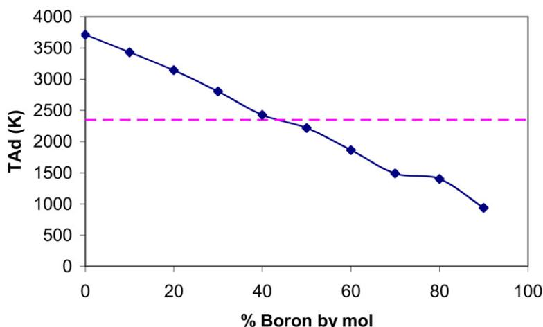
Fig. 3. Adiabatic flame temperature calculations for Al/B/CuO mixture. B is considered inert in these calculations. Boiling temperature of  $B_2O_3 = 2338$  K.
