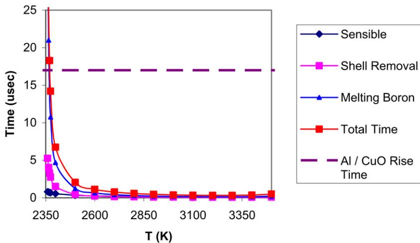
Fig. 6. Model predictions of the timescales as a function of surrounding temperature for a 700 nm boron particle.
