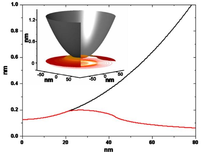
FIG. 2. (Color online) The line profile at the theoretical separation point of the silica sphere and silicon surface computed based on experimental data. The inset shows the representation of the contact obtained using the model.
