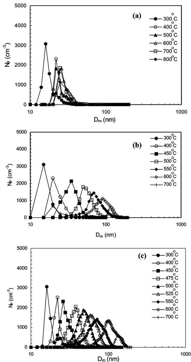
**Figure 5.** Temperature-dependent evolution of TDMA size distribution of carbon nanostructures grown on 15 nm Ni particles reacting with 5 SCCM  $C_2H_2$  and 100 SCCM  $H_2$  in the presence of (a) no oxidizer, (b) 150 ppm  $C_3H_6O$ , and (c) 200 ppm  $H_2O$ .
