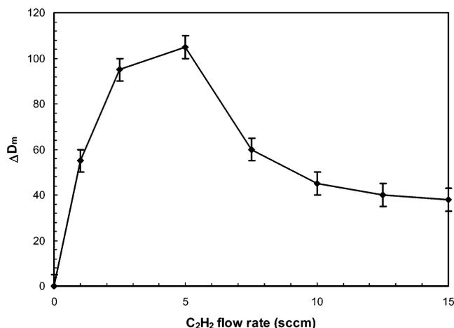
**Figure 6.** Mobility size change of carbon nanostructures as a function of the amount of  $C_2H_2$  addition on nickel particles selected by DMA-1.
