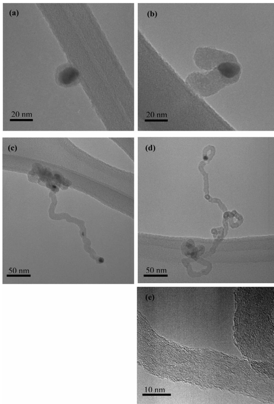
**Figure 3.** TEM images of gas-phase-grown carbon nanostructures collected at different temperatures (equivalent mobility size): (a) 400 °C ( $D_m = 28$  nm); (b) 450 °C ( $D_m = 44$  nm); (c) 500 °C ( $D_m = 70$  nm); (d) 600 °C ( $D_m = 120$  nm); (e) 600 °C ( $D_m = 120$  nm) [HRTEM]. [Experimental conditions: 5 SCCM  $C_2H_2$ , 50 SCCM  $H_2$ ].
