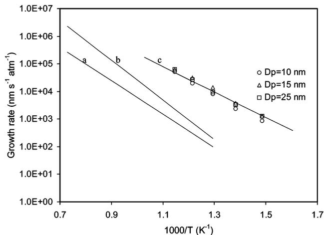
**Figure 8.** Growth rate comparison of this work, with selected prior studies (substrate-grown) as a function of temperature: (a) Ducati et al.,<sup>8</sup>  $E_a = 117$  kJ mol $^{-1}$ ; (b) Baker et al.,<sup>5</sup>  $E_a = 138$  kJ mol $^{-1}$ ; (c) current approach,  $E_a = 77 \pm 2$  kJ mol $^{-1}$ .
