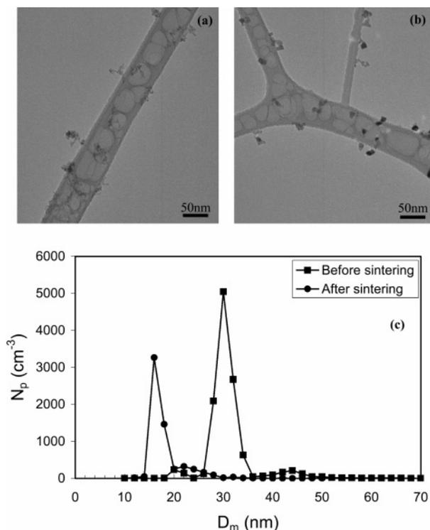
**Figure 2.** TEM images of 30 nm size-selected nickel particles (a) before and (b) after in-situ sintering process, and (c) TDMA size distribution measurement of the effect of sintering on 30 nm size selected particles.
