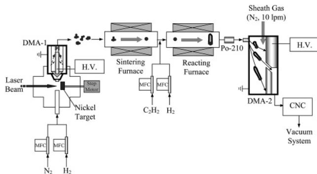
**Figure 1.** Schematic of laser ablation/tandem differential mobility system. DMA: differential mobility analyzer. CNC: condensation nucleus counter. MFC: mass flow controller. H.V.: high voltage power supply.
