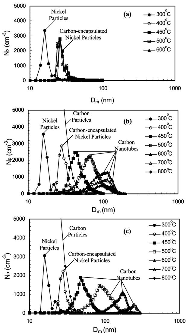
**Figure 4.** Temperature-dependent evolution of TDMA size distribution of carbon nanostructures grown on 15 nm Ni particles reacting with 5 SCCM  $C_2H_2$  and (a) 0 SCCM  $H_2$ , (b) 50 SCCM  $H_2$ , and (c) 100 SCCM  $H_2$ .
