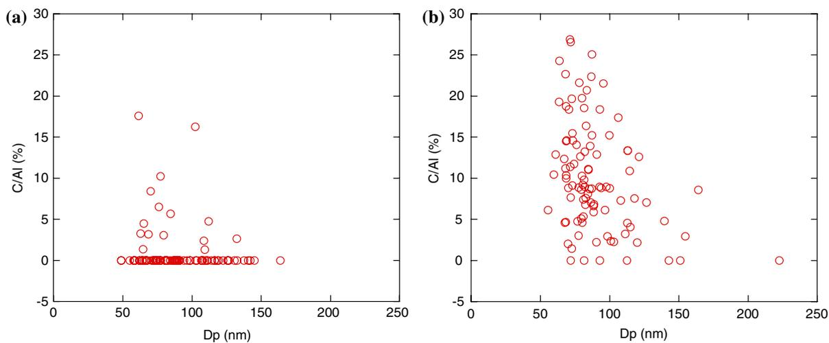
Figure 9. Elemental ratios of carbon to aluminum for the coated aluminum nanoparticles heated to 900°C after mixing with air (a) and heated in argon environment (no air) at the same condition (b).
