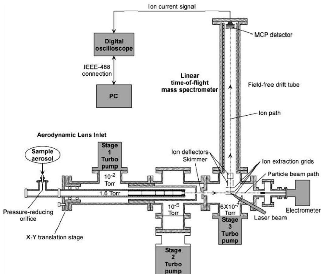
Figure 2. Schematic of Single Particle Mass Spectrometer.
