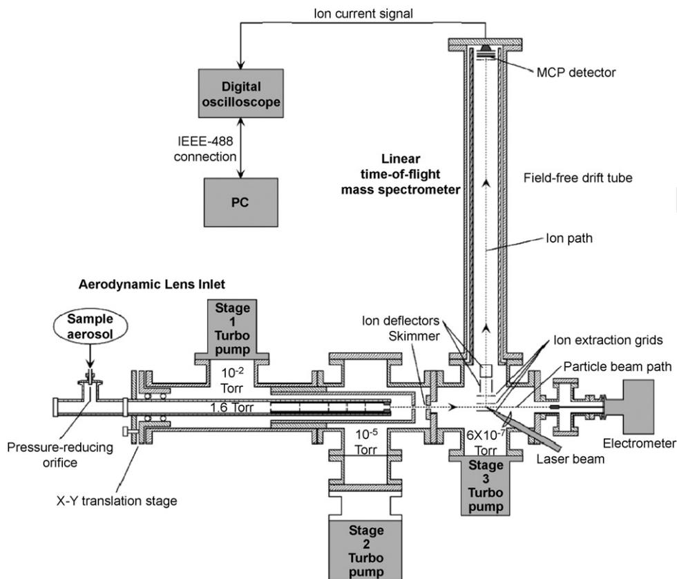
Fig. 1. Schematic of single-particle mass spectrometer (SPMS).
