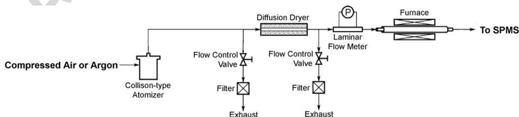
Fig. 2. Schematic of the particle generation system.
