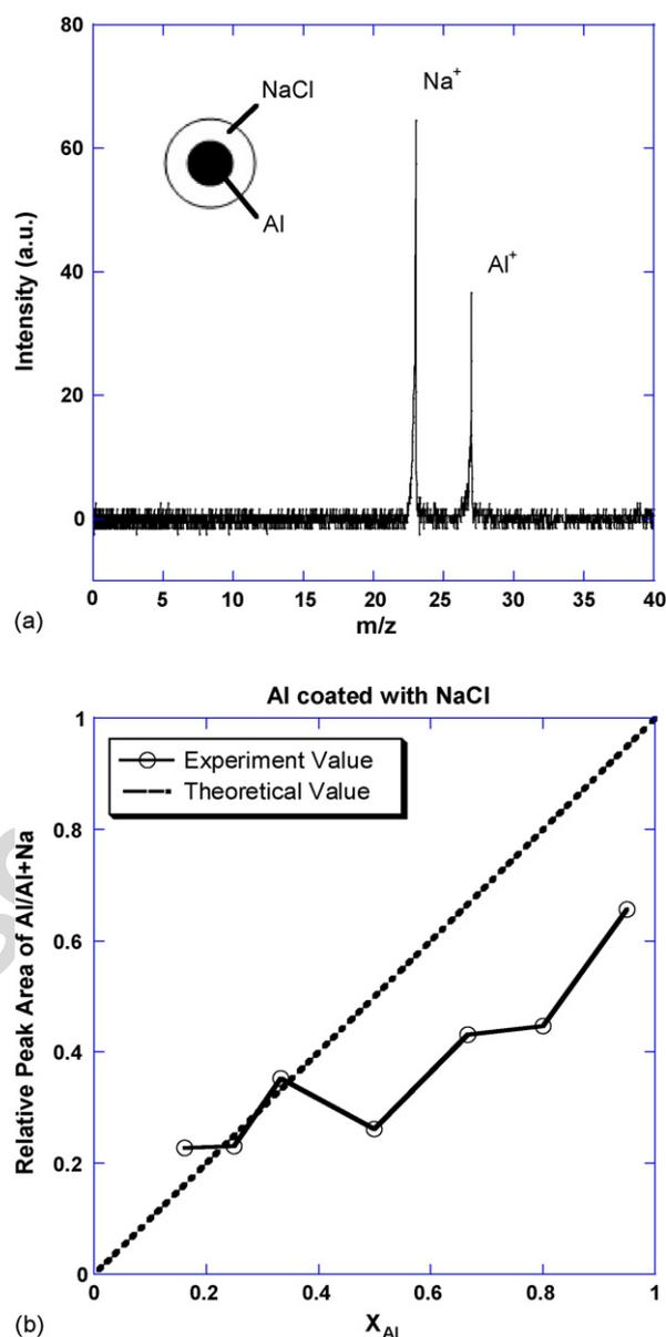
Fig. 4. (a) Typical mass spectrum of aluminum coated with NaCl (aluminum elemental mole fraction of  $X_{Al} = 0.95$ ) and (b) relative aluminum elemental mole fraction for aluminum particles coated with NaCl.
