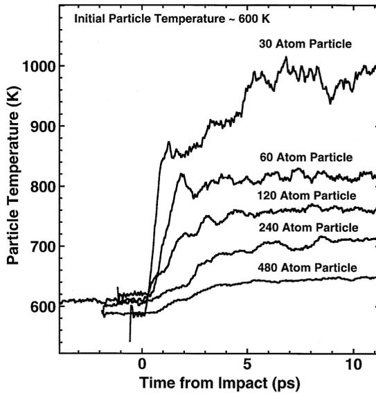
Fig. 4. Temporal evolution of particle temperature showing large initial temperature rise for very small particles.
