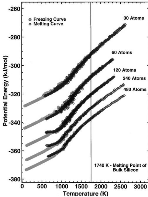
Fig. 7. Freezing and melting point curves as a function of particle size. This shows the range where the particles are all solid, all liquid or a mix of both. The freezing point curve is gray and the melting point curve is black.
