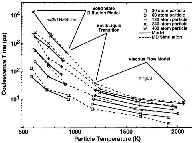
Fig. 8. Coalescence times as a function of particle size and temperature. Dotted lines connect the MD computations. The solid curves represent the viscous and solid state diffusion models. Note: The model results for the liquid phase were increased by a factor of ten so they would line up with the MD simulations.
