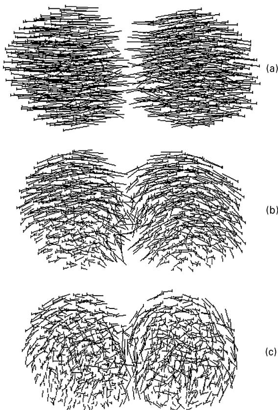
Fig. 5. Time series of particle morphology imaged with respect to atomic velocity vectors for two 480-atom particles at 900 K.
