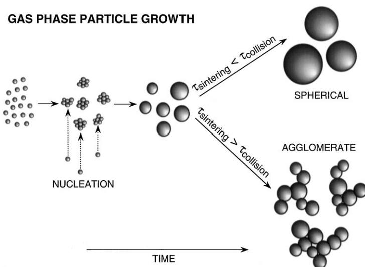
Fig. 1. Temporal evolution of vapor-phase particle growth.
