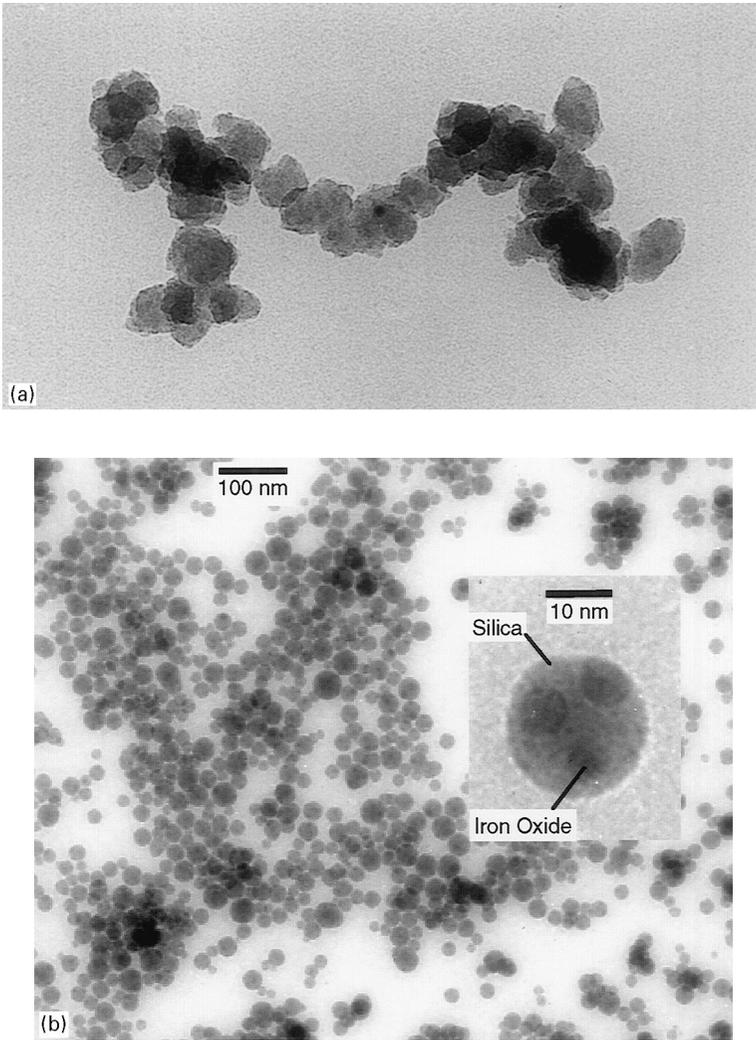
Fig. 2. Examples of agglomerates and spherical nanoparticles formed from vapor phase growth. (a) agglomerate of  $\text{SiO}_2$ , (b) spherical superparamagnetic nanocomposite of  $\text{SiO}_2/\gamma\text{-Fe}_2\text{O}_3$  (Zachariah *et al.*, 1996b).
