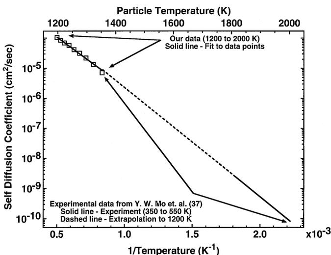
Fig. 6. Computed silicon self-diffusion coefficients. This plot contains our results at high temperatures (1200–2000 K) and the low temperature (350–550 K) experimental data of Mo *et al.* (1992). The dotted line is an extrapolation of Mo's data to 1200 K.
