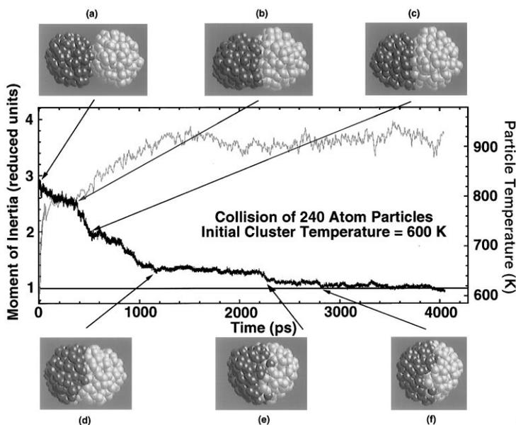
Fig. 3. Temporal behavior of particle morphology as a function of temperature for the collision of two 240-atom particles. The gray curve is temperature. The black curve is the reduced moment of inertia.
