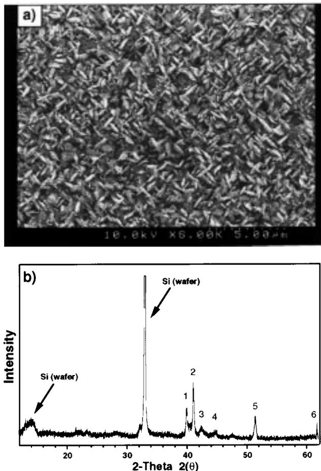
**Figure 6.** (a) SEM image of sample R22 grown on Si(100) at 600 °C showing two preferred growth orientations orthogonal to each other. (b) XRD spectrum of sample showing that titanium silicides ( $Ti_xSi_y$ ) have formed. At 600 °C, the deposited Ti reacted with the silicon substrate to form titanium silicides, as has been previously reported in the literature.<sup>20</sup> See Table 2 for identification of the numbered peaks.
