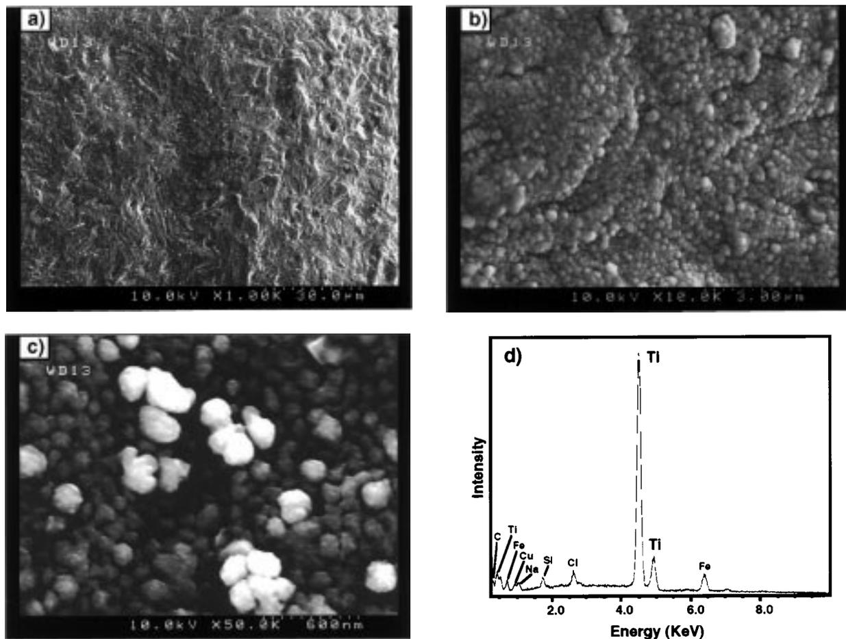
**Figure 7.** SEM images of sample R26 (grown on OFHC copper substrate at 610 °C) taken at (a) image magnification of 1000; (b) image magnification of 10 000; (c) image magnification of 50 000; (d) EDS spectrum of film shows clearly the presence of titanium, trace signals of Cu, Na, Si, Cl and Fe, and no oxygen signal.<sup>23</sup> The Cu signal is from the substrate and the weakness of the signal is due to the titanium overlayer. An EDS beam energy of 10 keV was used.
