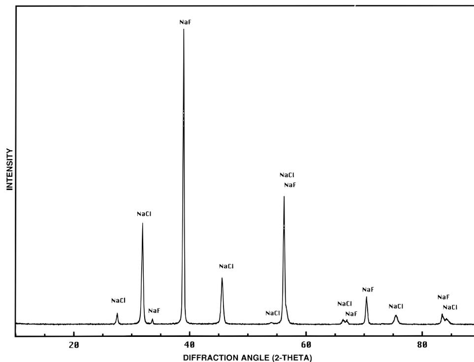
FIGURE 4. Example of X-ray diffraction pattern of products of reaction.
