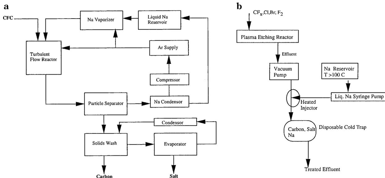
FIGURE 6. Schematic of a potential closed-loop Na/CFC aerosol mineralizer.
