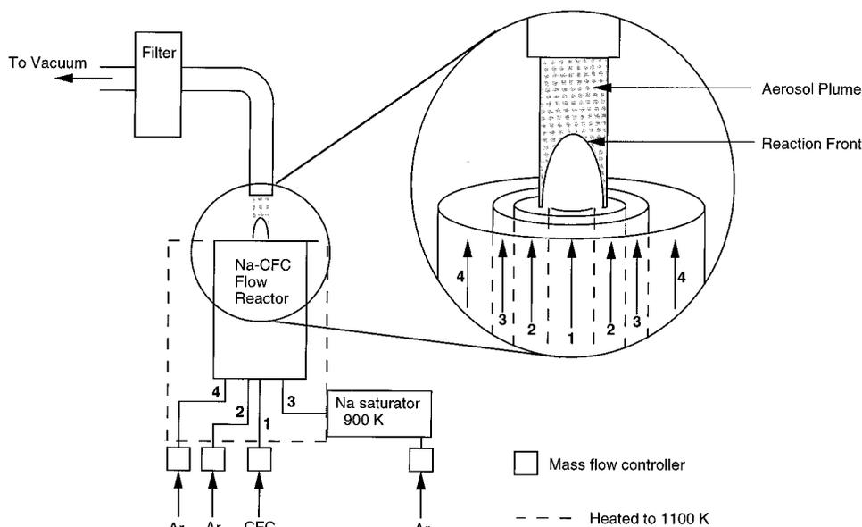
FIGURE 2. Schematic of Na/CFC reactor.
