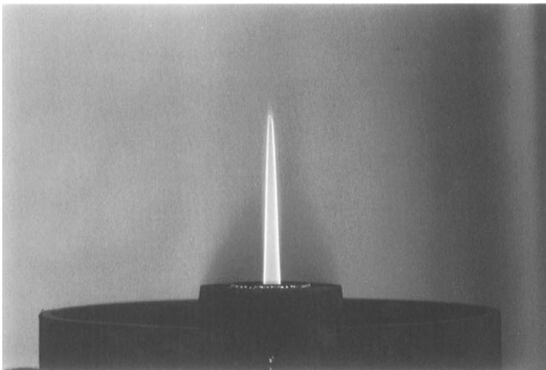
FIGURE 3. Photograph of reaction zone for  $\text{CF}_3\text{Cl} + \text{Na}$ .
